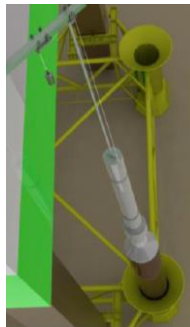
Figure 5 Hammer positioned on pile
