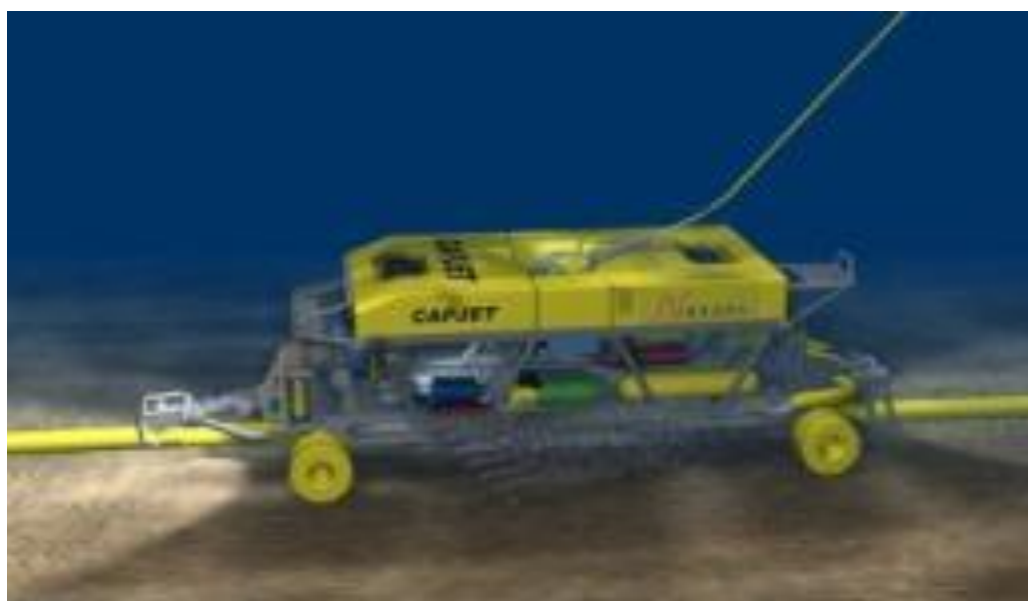
Fig 2. The Capjet trenching machine
