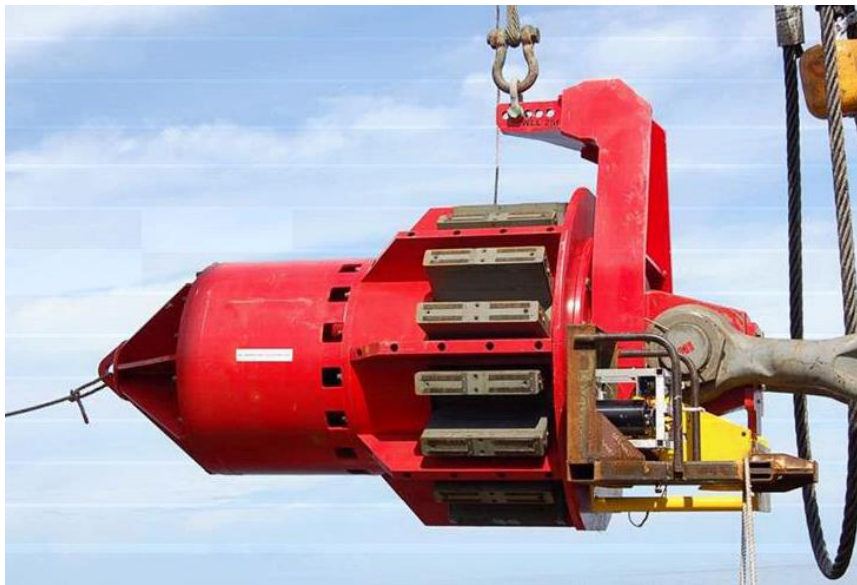
Fig 4 ILT – Internal Lifting Tool – used to stab and lift piles
