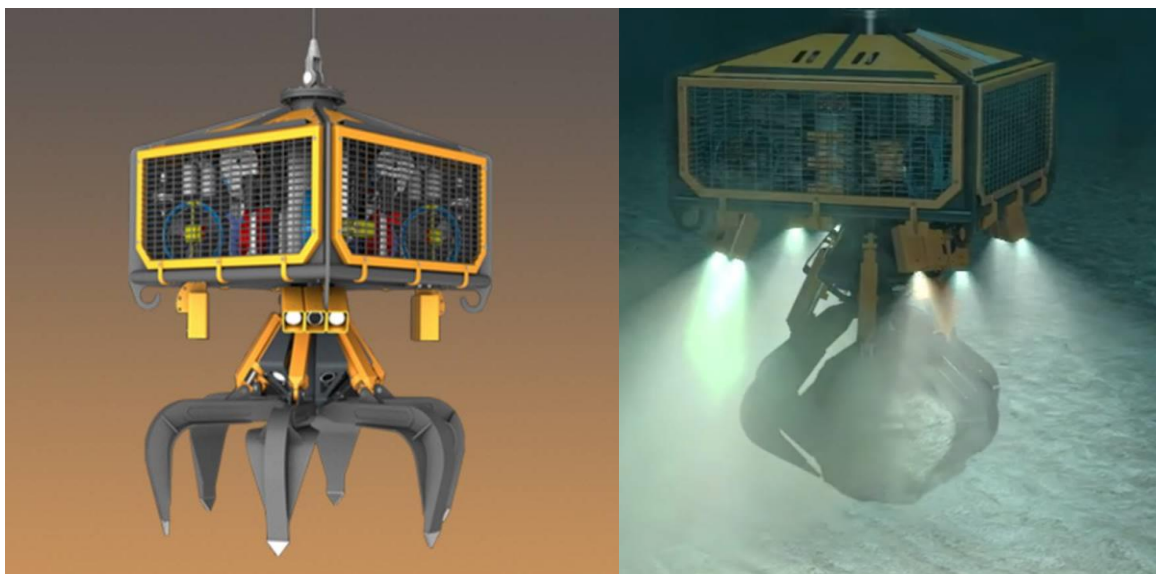
Fig 3 UTROV Grabber system for boulder removal
