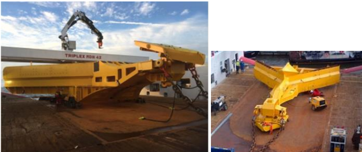
Fig 2 Ecosse Subsea Systems 15m SCAR Plough
